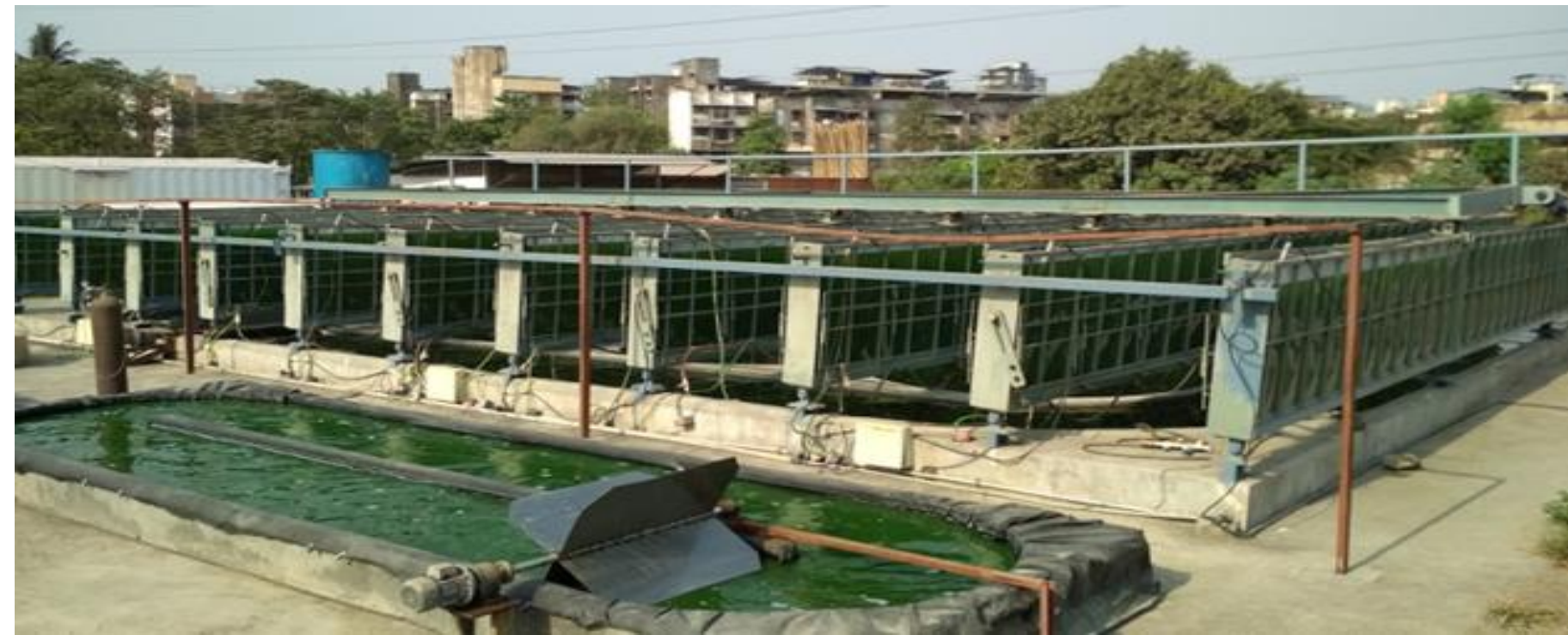
Marine algae cultivation In Mumbai coast in 100,000 liter scale specially designed photobioreactor
